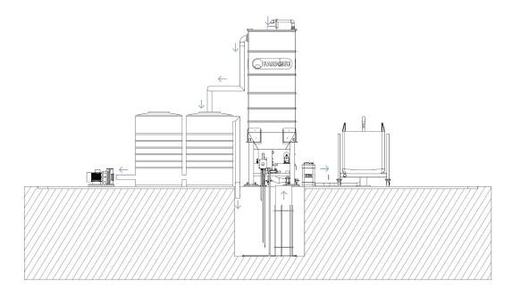
Ideal for the smaller factory, the **SILO 2500** is a compact system for the quick removal of mud from your recycled water.
